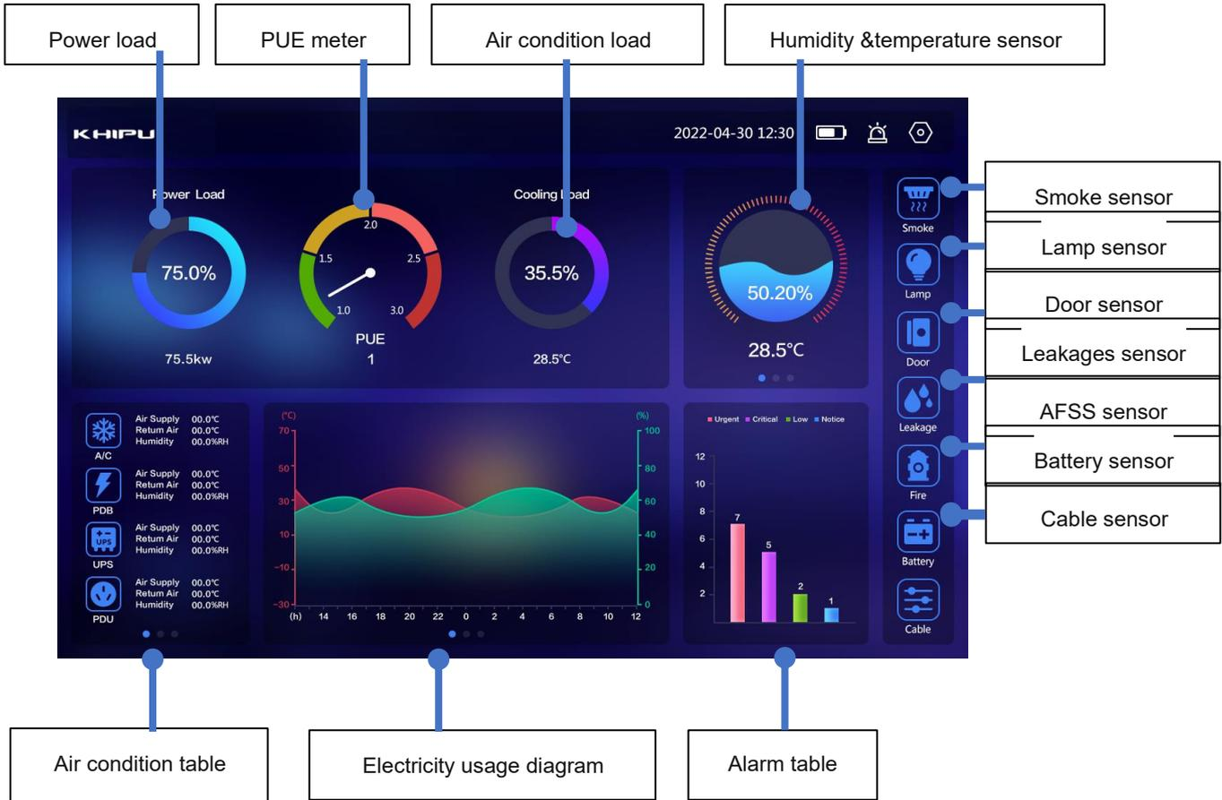
UPS: Collect the main circuit, bypass power quality such as voltage, current, power, frequency, and other information; At the same time, the operating state of the equipment is also monitored, such as UPS on/off state, operation mode and power supply mode, and the working state of its internal key electrical units.
