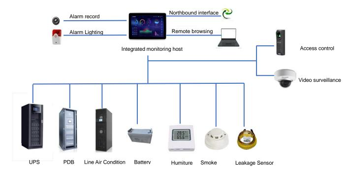
Dynamic environmental monitoring system is a centralized monitoring of power equipment and environmental variables in all kinds of computer rooms.
